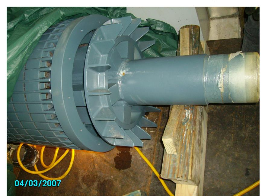
Sister rotor, non-identical design (used with the same stator / frame, but OEM redesigned the rotor – this is a different generation)
