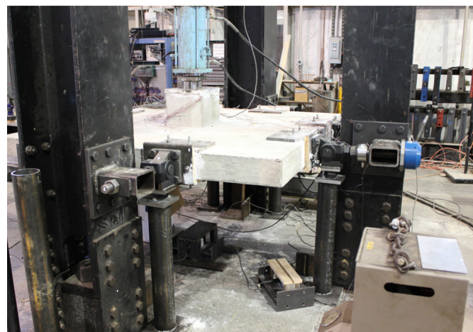
Fig. 8. Test setup for slab-column connections subjected to in-plane restraints
