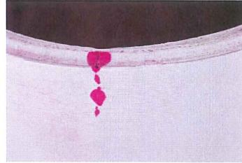
capillary action, which is caused by intermolecular forces. In this case the capillary action occurs when the combination of the surface tension of the liquid penetrant and the adhesive forces of the walls of the crack work together to cause the liquid to climb and color the developer.
