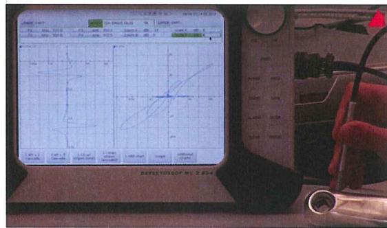
*A crack is detected in the part. Screenshot courtesy of \_*
