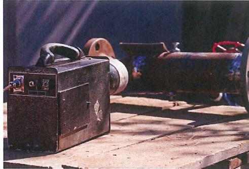
*Radiographic testing of a welded joint*
