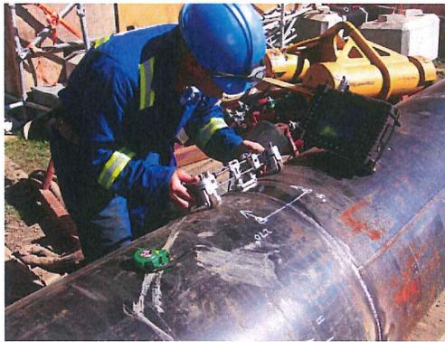
*Ultrasonic testing of a pipeline weld*
