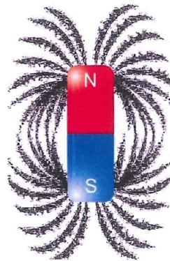
*Iron particles concentrated along magnetic field lines*
