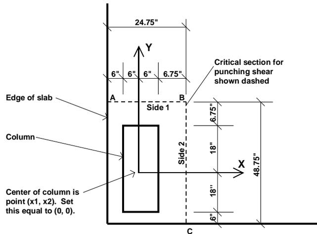
Figure 8: Corner Column, Point 5 in SAFE Model
