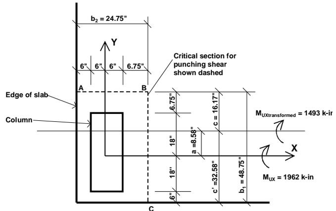
Figure 15: Corner Column, Point 5 in SAFE Model
