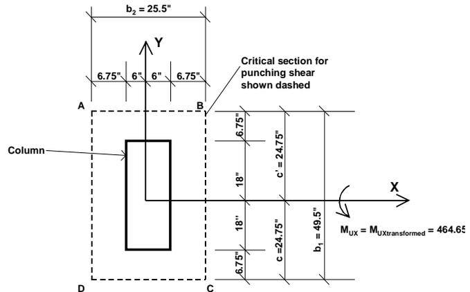
Figure 9: Interior Column, Point 10 in SAFE Model
