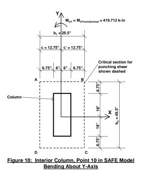
$$\frac{J_Y}{c_Y} = \frac{b_1 d(b_1 + 3b_2) + d^3}{3} = \frac{25.5 \times 13.5(25.5 + (3 \times 49.5)) + 13.5^3}{3} = 20786.6 \text{ in}^3$$
