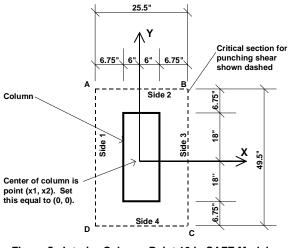
Figure 5: Interior Column, Point 10 in SAFE Model
