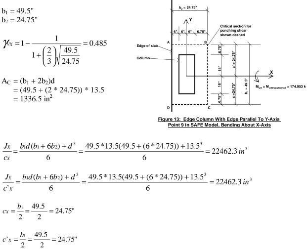
$M_{UXtransformed} = M_{UX} = 174.953$  k-in (direction of moment shown in Figure 13)
