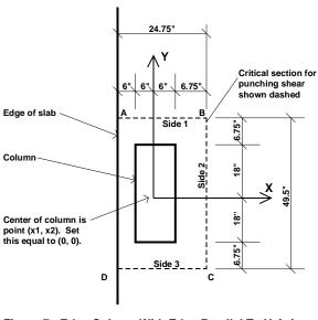
Figure 7: Edge Column With Edge Parallel To Y-Axis, Point 9 in SAFE Model
