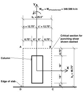
Figure 12: Edge Column With Edge Parallel To X-Axis Point 6 in SAFE Model, Bending About Y-Axis
