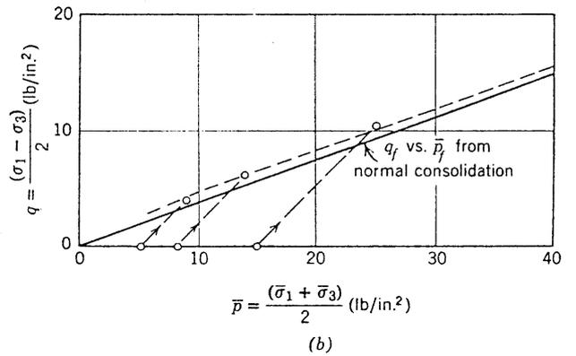
Fig. 21.5 Results of CD tests on overconsolidated Weald clay.  $\bar{p}_m = 120$  lb/in.<sup>2</sup>
