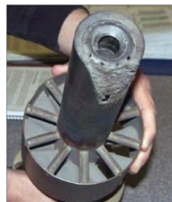
Figure 6: Flashback damage to a fuel nozzle 15 .
