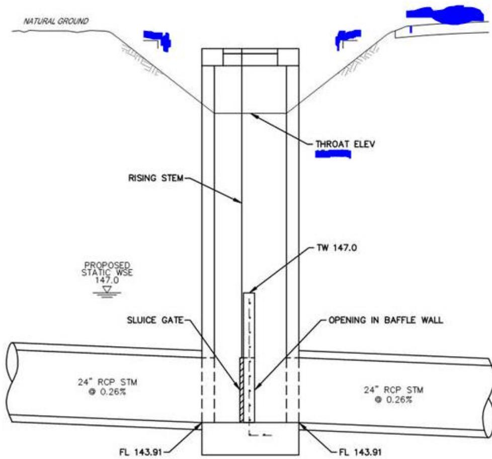
**INLET W/ BAFFLE WALL DETAIL**
