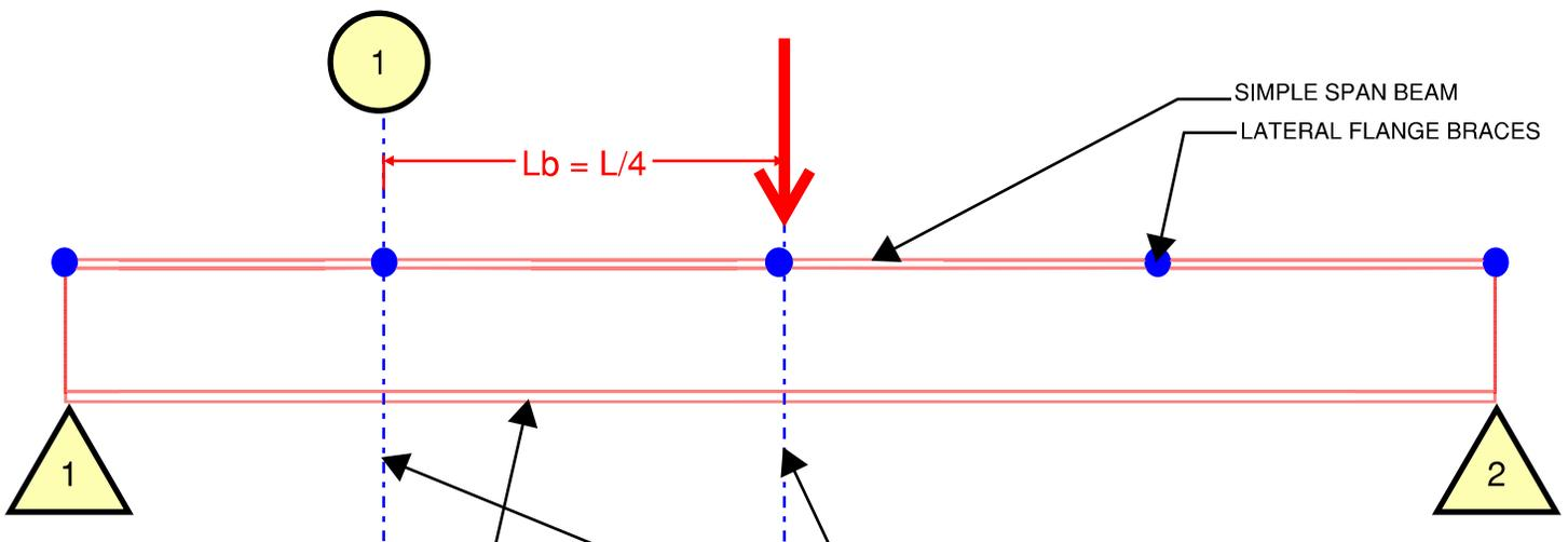
PERHAPS WE ASSUME THAT THE BOTTOM FLANGE SPANNING AS A GIRT TO THE SUPPORTS PROVIDES ROTATIONAL RESTRAINT TO SECTIONS ONE AND TWO WHEN THERE IS NO BOT FLANGE COMPRESSION? AND NEGATIVE LTB CHECKING COULD SORT OF SERVE AS A WAY TO ENSURE THAT THE BOTTOM FLANGE CAN STILL DO THIS JOB WHEN UNDER COMPRESSION?
