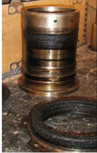
Physical damage to the bellows and seal faces was not visible, however this does not conclude that there is no damage present. The deposits were dry at the time of inspection it is not known if at the time of removal from the pump the deposits were actually sticky. There may be implications on seal integrity and life if this is found to be the case. Further inspection by John Crane is required to fully assess the condition of the mechanical seal components.
