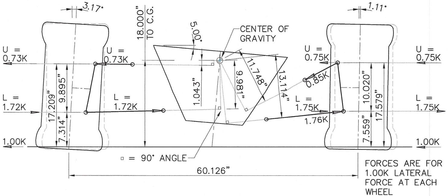
CHASSIS ROLL FORCE EACH SIDE FROM 1.0 K UNIT LOAD EACH WHEEL:
