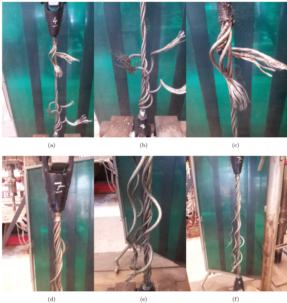
FIGURE 5.3: Photographs test specimen (a) (b) (c) specimen number 4, d=14 mm (d) (e) (f) specimen number 7, d=20 mm
