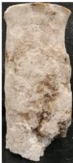
Figure D-3. Specimens deformed at 3000-psi chamber pressure (Photo courtesy of Thai Nguyen)
