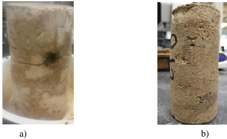
Figure 6-18. Outlier extension test specimens: a) Hole on specimen, b) One end of specimen is much softer (Photo courtesy of Thai Nguyen)
