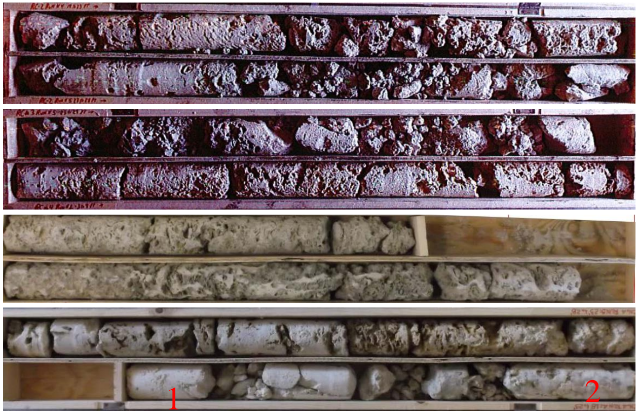
Figure 2-6. Examples of core runs with low RQD (Photo courtesy: Thai Nguyen)
