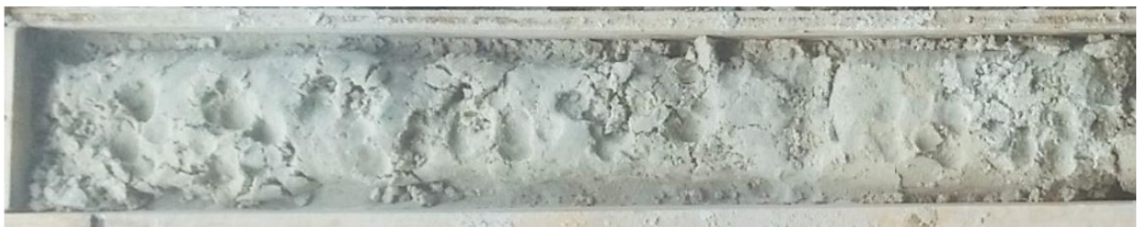
Figure 2-5. Weak poorly cemented silt, sand, limestone mixture in a core run (Photo courtesy: Thai Nguyen)
