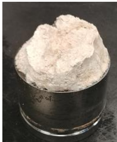
Figure D-3. Specimens deformed at 3000-psi chamber pressure (Photo courtesy of Thai Nguyen)
