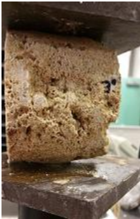
Figure 3-10. BST on sample 624-3 with uneven diameter (Photo courtesy of Thai Nguyen)
