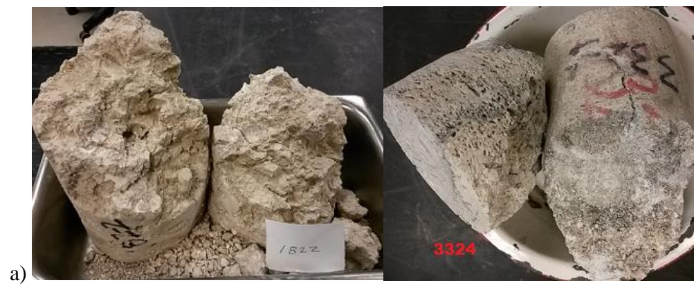
Figure D-2. Specimens tested at 130-psi chamber pressure: a) \gamma_{dt} > 130 pcf (Photo courtesy of Thai Nguyen)
