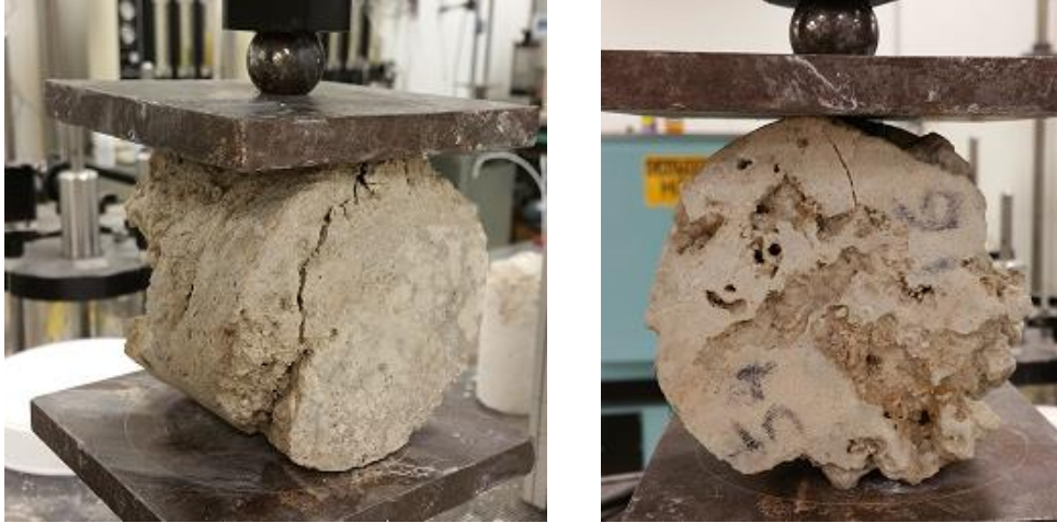
Figure 3-7. Non-center splitting - BST tests on samples 534-1 and 541-6 (Photo courtesy of Thai Nguyen)
