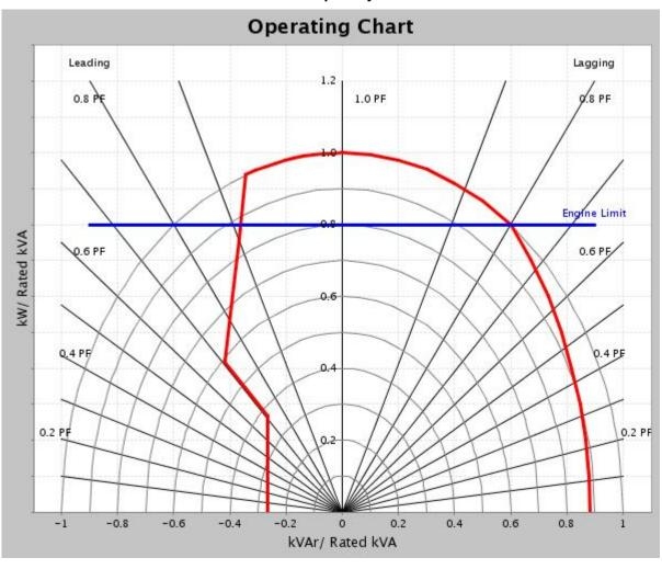
Engine: 3516 Generator Frame: 825 Genset Rating (kW): 1825.0 Line Voltage: 480
