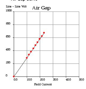
Engine: 3516 Generator Frame: 825 Genset Rating (kW): 1825.0 Line Voltage: 480
