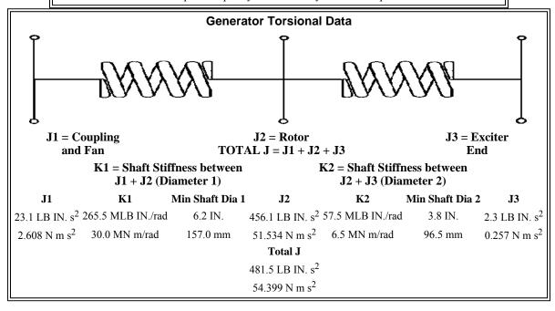
Engine: 3516 Generator Frame: 825 Genset Rating (kW): 1825.0 Line Voltage: 480
