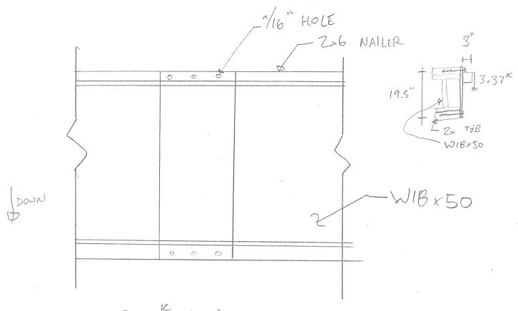
$$T/c = \frac{3.37^{k} \times 3^{"}}{19.5^{"}} = 0.518^{k}/3 \text{ bolts} = 173 \frac{\#}{Bolt} \text{ Tension}$$
