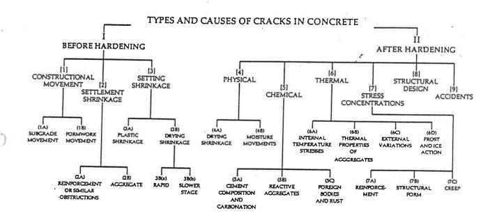
Figure 1 - Causes of Cracking in Concrete
