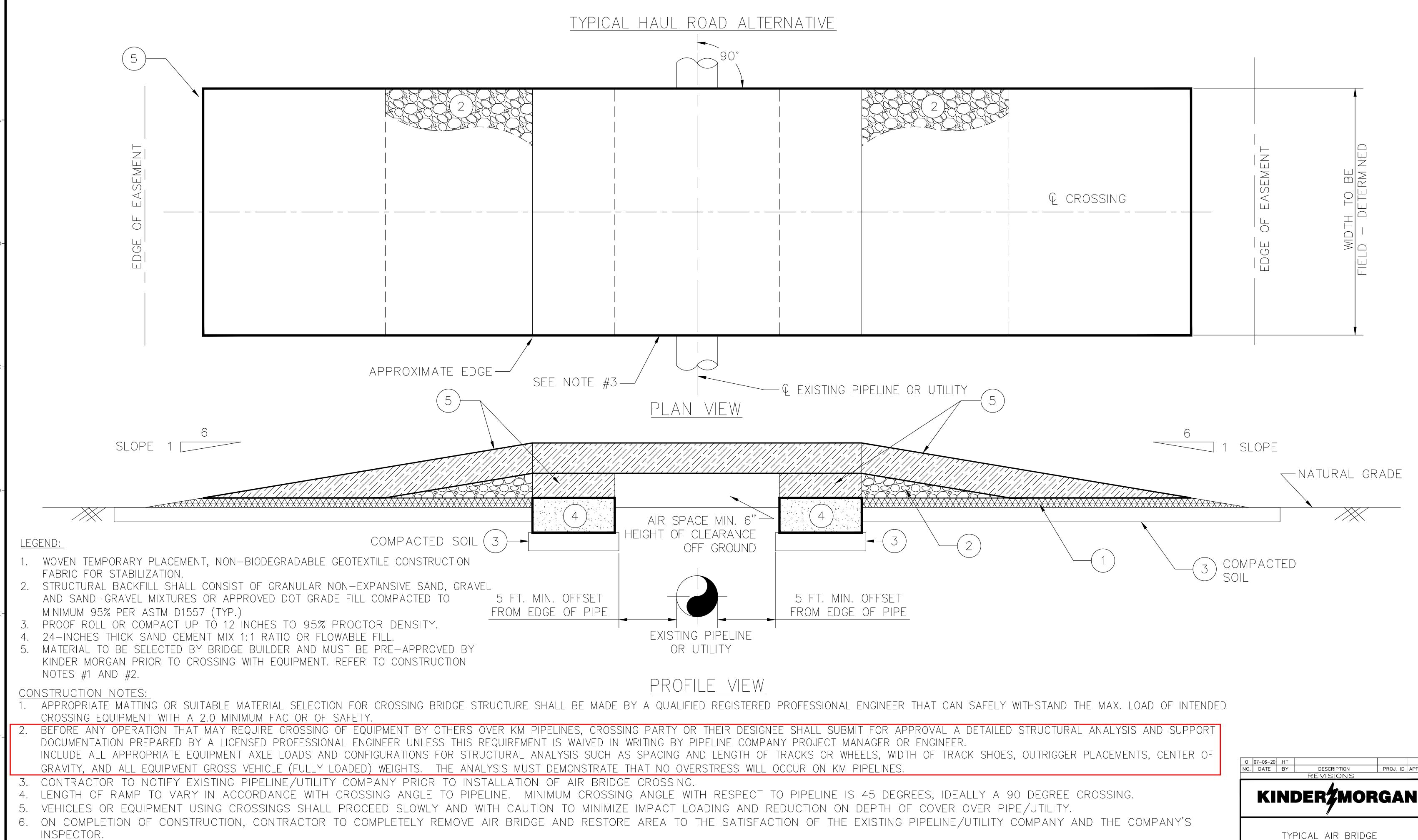
8. IN LIEU OF COMPACTION AND PROOF ROLLING, A 4 — INCH THICK WOODEN MATS MAY BE USED ON OTHER SIDE OF THE PIPELINE IN CASE CERTAIN EQUIPMENT CANNOT CROSS THE PIPELINE DUE TO STRESS LIMITATIONS.
