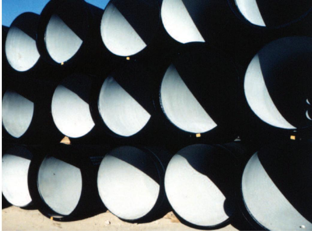
Cement-mortar linings have been applied to Gray Iron and Ductile Iron pipe for more than 82 years. DIPRA is not aware of any performance problems that have occurred due to cracks or loose cement-mortar linings as long as the lining was intact before placing the line in service.
