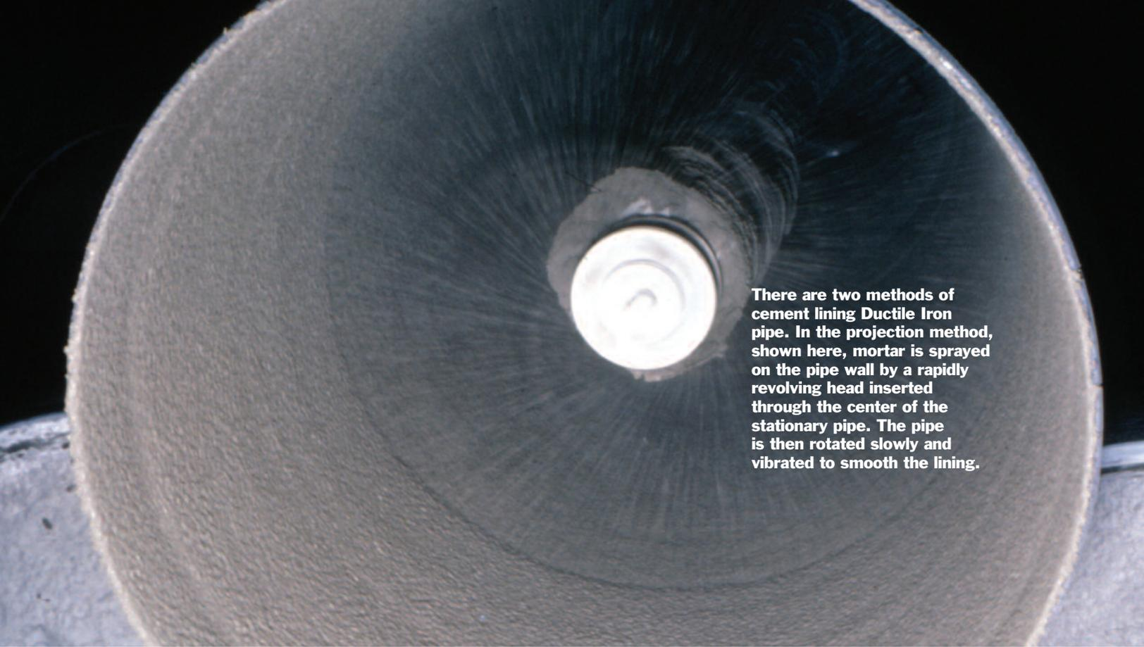
**There are two methods of cement lining Ductile Iron pipe. In the projection method, shown here, mortar is sprayed on the pipe wall by a rapidly revolving head inserted through the center of the stationary pipe. The pipe is then rotated slowly and vibrated to smooth the lining.**
