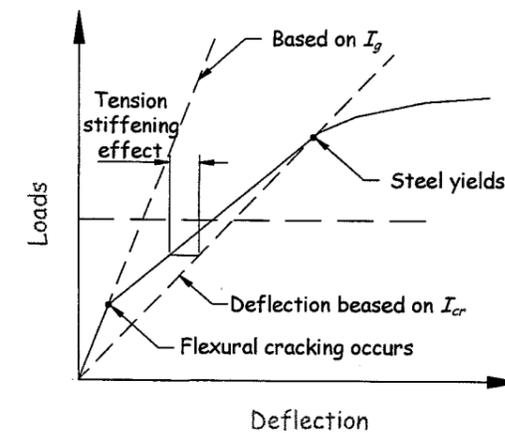
The value of  $I_e$  varies with the stress level in the beam. It is greater than  $I_{cr}$  to allow for tension stiffening effects, as discussed earlier. In the New Zealand code the effective moment of inertia is given by (see 3.3.2.3):
